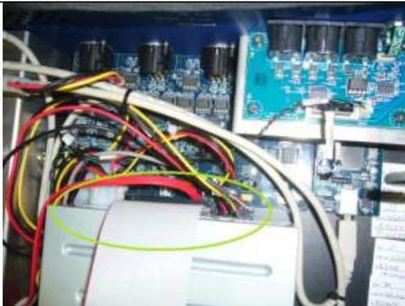
4. Disconnect the cables from the CD drive and the hard drive. Hard drive is located beneath the CD drive. Both drives are mounted in the same retainer. The CD drive has 3 connections and the HDD has 2 connections.
