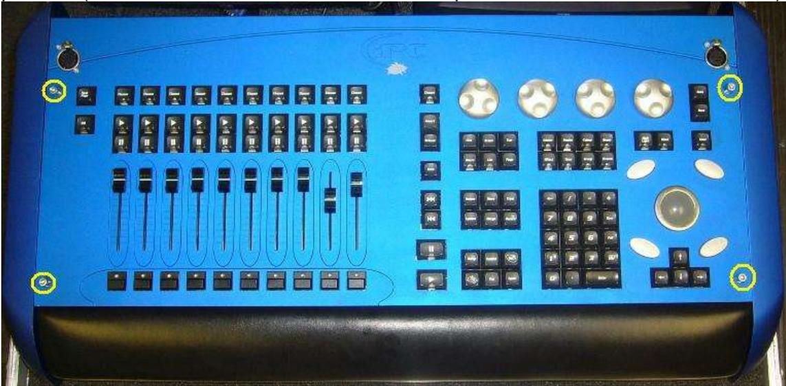
2. Gently lift the front panel PCB (circuit board) up as you would a car hood (there are connections at the top of this board that can be damaged if you pull straight up). Please note this circuit board is not hinged to the console.
