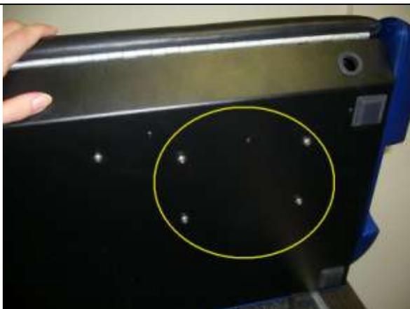
5. To remove the HDD/CD drive retainer, carefully raise the console up and remove the 4 screws on the right half of the underside of the desk. Use caution so that the drives do not fall out, or cause damage to the other PCBs inside the console.
