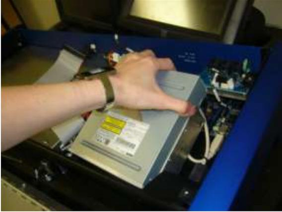
6. Remove the CD drive and HDD from the console carefully.
